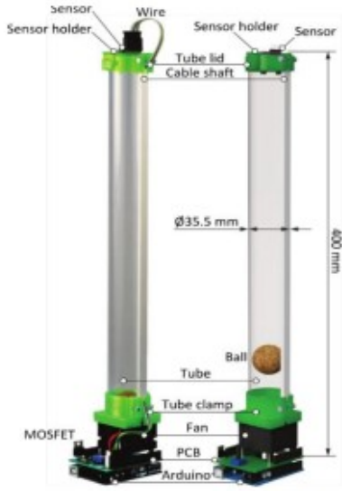
Fig. 1. Floatshield laboratory plant, Takács et al. (2020).
